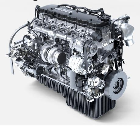
The 6.7 litre Euro 6 PACCAR PX-7 engine uses ultra-modern common rail technology, a highly optimised fixed geometry turbo with wastegate, exhaust throttle and air intake throttle. In order to comply with the strict Euro 6 emissions requirements, SCR technology and an active soot filter.
